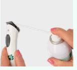
An oil spray with a small tube attachment is well suited for cleaning and oiling between the shearing blades. This creates more pressure and the dirt is blown out and the oil can be better distributed between the shearing blades.
